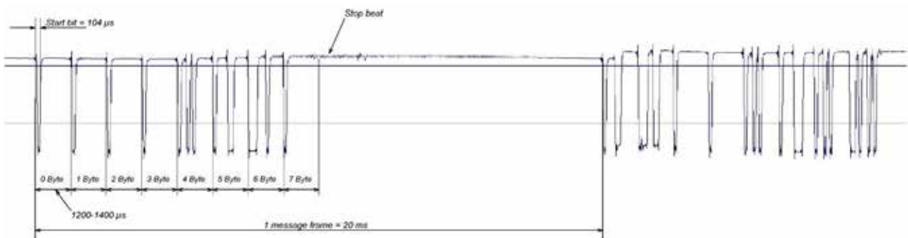
Fig. 5. General view of the timing diagram of the LANC protocol
