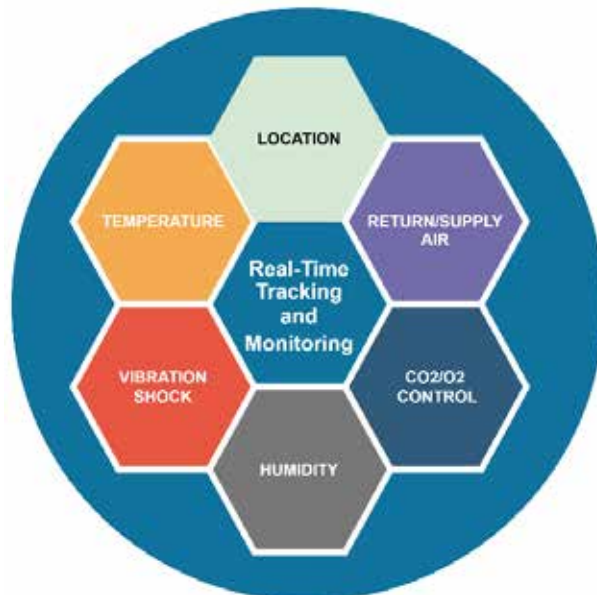
Fig. 3. Container IoT sensors data output
